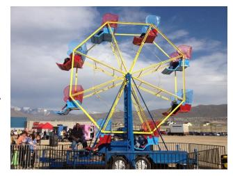
rebuilt, some using water ballast instead of the permanent foundations of their fixed counterparts.
