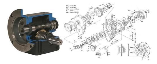
An Example of a Reduction Gearbox and Assembly drawing that may be used in this part of the competition.
