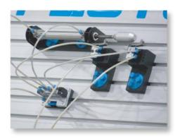
Example of Festo Didactic components that competitors will use to design, build and troubleshoot a Multi Cylinder Sequential or Cascade Circuit
