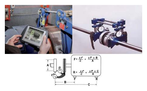
Example of Coupling / Shaft Alignment Project Dial Indicator or Laser (Fixturlaser NXA Pro) alignment equipment will be used by the competitor to complete the above task
