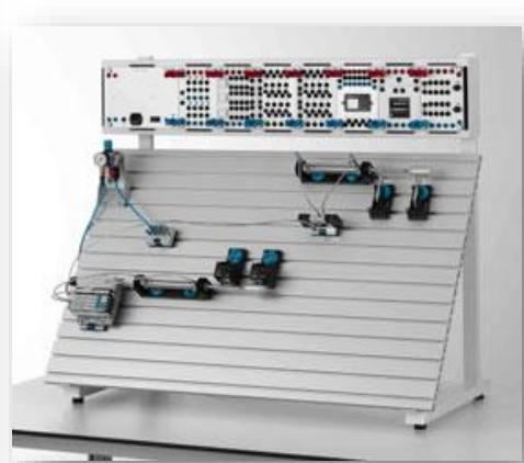
**Example's of Festo Didactic components that competitors may use to **design, build** and test the function a Multi Cylinder Sequential or Cascade Circuit.**
