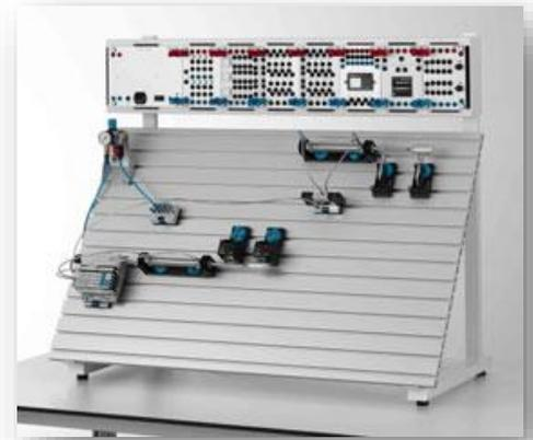
**Example's of Festo Didactic components that competitors may use to design, build and test the function a Multi Cylinder Sequential or Cascade Circuit that may include time-delay, flow control and / or check valves.**
