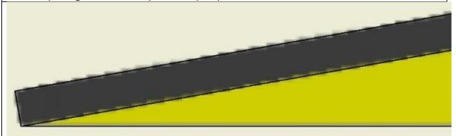
• These Straight Edge Cuts result in a 0.5 in. Tall Sloped Edge where the Ramp Cap meets the Court Floor.
