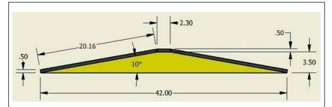
• The Ramp runs Side to Side in One Passageway and the Two Sided Ramp's Details are provided in the Appendix Section of this document.
