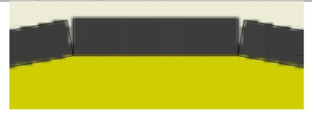
• The Ramp Slope and Top Caps ALL have Straight Edge Cuts. This results in a small Opening where the Slope and Top Caps meet.
